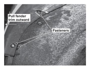
2. Remove the engine compartment cover by removing the twelve outer fasteners, six of which are pointed out below.
