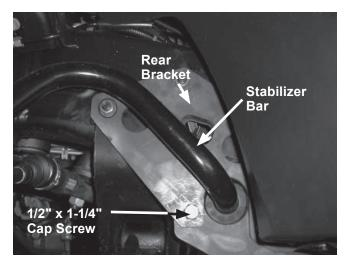
3. Insert a 1/2" x 1-3/4" cap screw and washer through the rectangular opening in the inner surface of the frame, through the frame and the rear bracket. Secure loosely with a 1/2" locknut. Adjust the position of the rear brackets upwards as far as possible and secure the 1-3/4" fastener, as well as the three 1-1/4" cap screws from Step 3.
