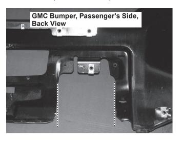
Remove the plastic portion of the bumper and notch as shown below.
