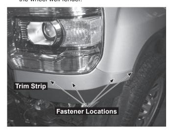
6. Remove the fastener to the side of the plastic trim piece. Remove the trim piece.
