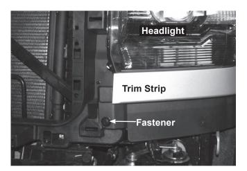
7. Remove the two fasteners on the underside of the headlamp trim.
