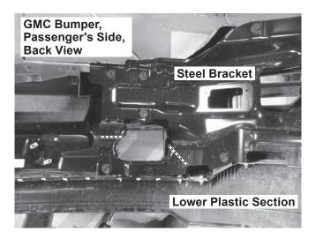
2. Notch to create an opening in the tow hook cavity in the steel portion of the bumper.
