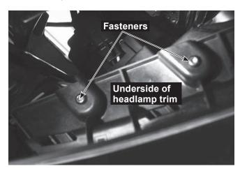
8. The headlamp is held in place by four fasteners. Remove the two fasteners on the top of the headlamp, as well as the fasteners on the side and the front.
