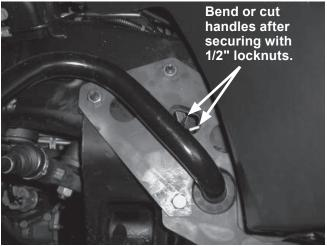
Repeat this process on the driver's side, noting that the rearmost cap screw on handle must be inserted through the round hole behind the rear bracket as shown. Bend or cut handles so that they do not interfere with the range of motion of the front stabilizer bar.
